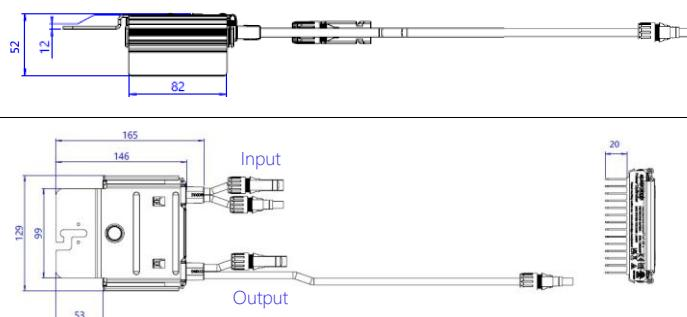
\* When installing SolarEdge power optimizers, maintaining clearance is required. Refer to the [Power Optimizer Clearance Application Note](#) for more details.
